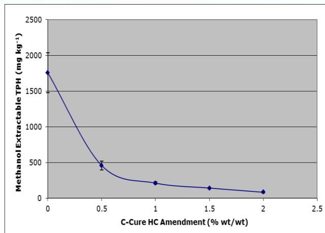
*Figure 1. Concentrations (mg/kg) of methanol extractable hydrocarbons (TPH) in drill cuttings stored in a lined pit. Drill cuttings were treated with different amounts of C-Cure product to reduce leachable hydrocarbons. Data are presented as averages ± standard error of the mean.*
