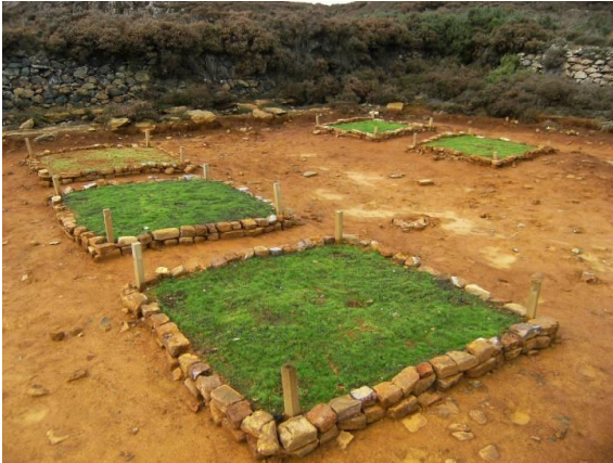
Figure 4b: Plots treated with C-Cure metal+ showing restoration of plant growth on heavy metal impacted sediment at the Parys Mountain mine site.
