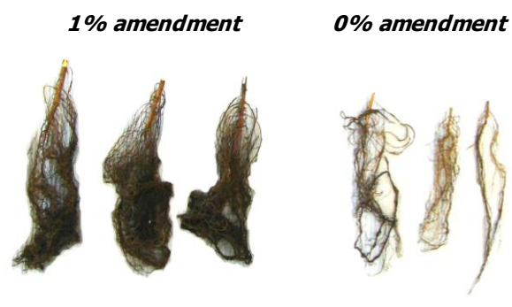
Figure 2: Root development in mine tailings treated with 1% (wt/wt) C-Cure-Metal compared to un-amended control.
